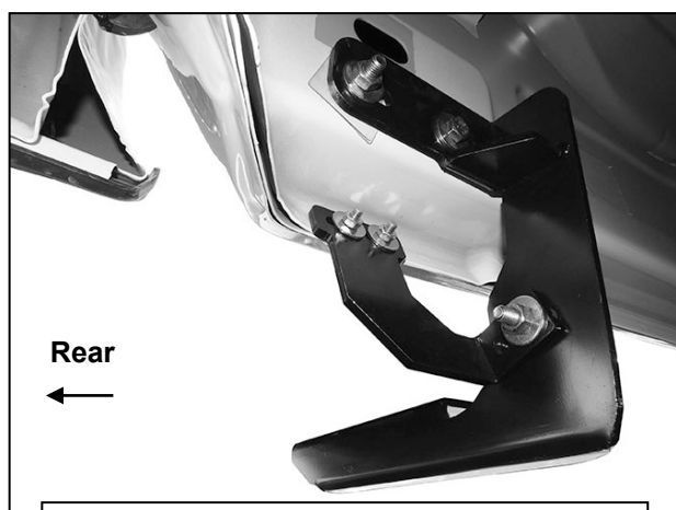
(Fig 15) Driver/Left rear Brackets installed
