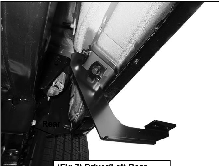
(Fig 7) Driver/Left Rear Mounting Bracket installed
